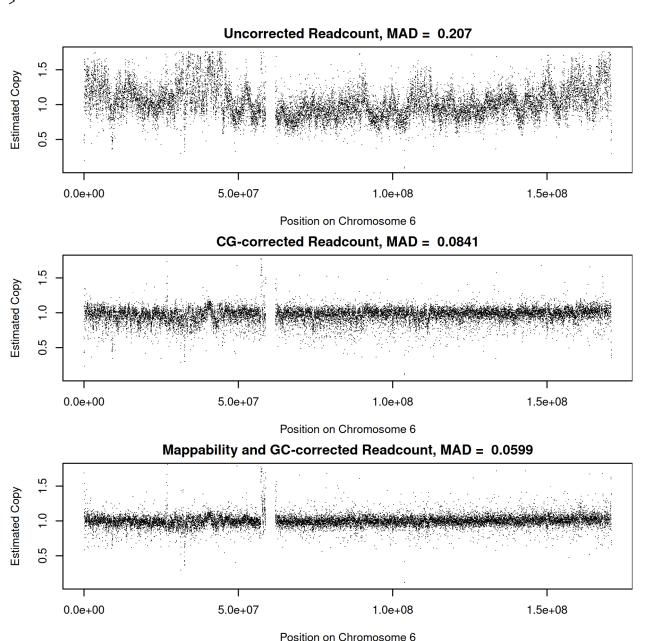
In the top track, the original uncorrected reads are used to estimate copy number (by simply dividing by the median value), followed by tracks with additional GC then mappability correction. Mediam absolute deviations (MAD) measuring the variance of each track can be seen to decrease after each correction step.
