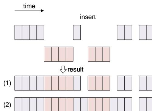
Figure 6.1: Insert operation for temporal values.
