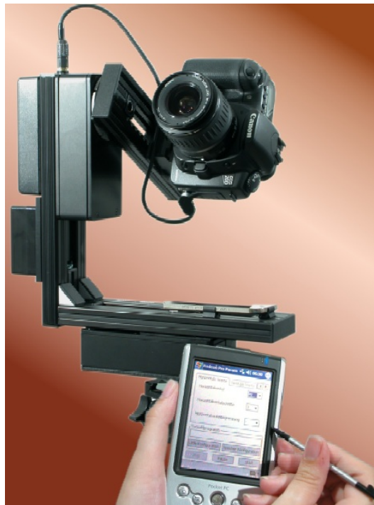
Figure 7.4: Automated panorama head. (Source: Wikipedia https://commons.wikimedia.org/wiki/File:Rodeon_vr_head_01.jpg )
